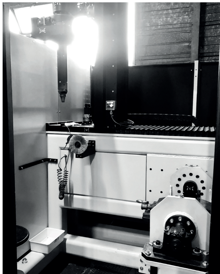
PTA torch overall view used on full cavity coated moulds
