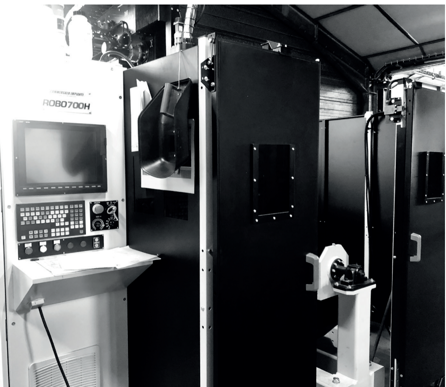
CNC controlled PTA welding equipment used on full cavity coated moulds
